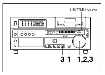
1 Press the SEARCH button or search dial so that the SHUTTLE indicator in the display section is lit.
